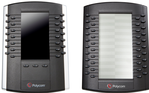
Figure 2: Expansion Module LCD color display and paper display
